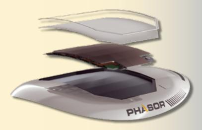
Phasor's system is unique — proprietary microchips (or ASICs) control each of these tiny patch antennas — this unique system architecture can combine signals more efficiently and effectively to maximize gain. A dynamic, software-controlled antenna is created that can quickly and robustly track any satellite through a closed-loop feedback algorithm.
